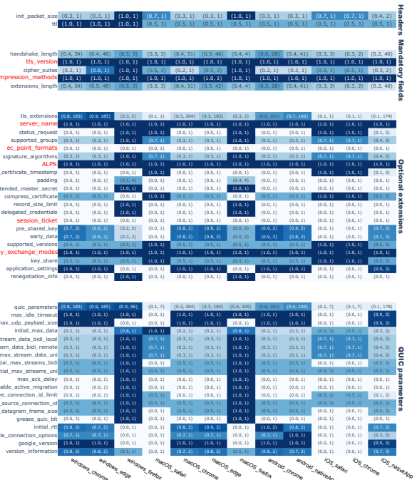
(a) Handshake field values of YouTube flows over QUIC across 12 user platforms.
