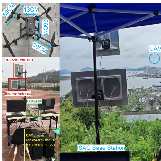
Fig. 9: UAV micro-Doppler extraction test scenario based on ISAC hardware testbed.
