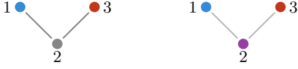
FIG. 16. Two cases for the local connectivity for the interaction terms. The blue and red qubits correspond to the physical up and down states, the purple sites are the secondary qubits, and the grey are ancilla.
