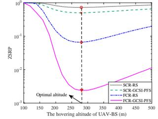
Fig. 4. The ZSRP versus the hovering altitude of UAV-BS.
