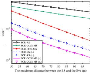
Fig. 2. The ZSRP versus the maximum distance between the UAV-BS and the Eve, where “t,” and “s,” stand for theoretical and simulation results, respectively.
