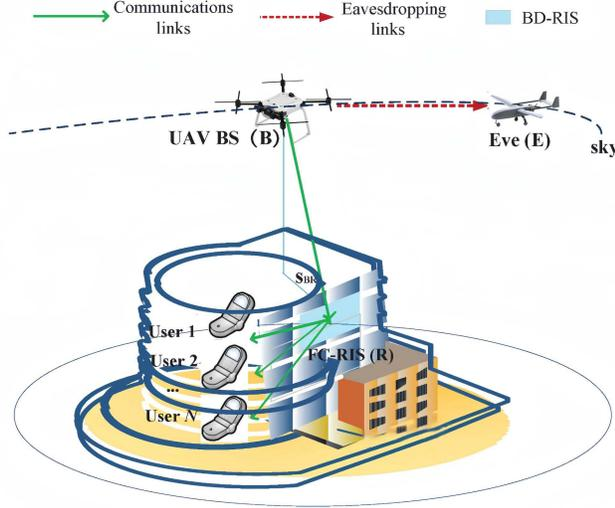
Fig. 1. The considered FC-RIS and UAV aided multiuser communications network in the presence of an aerial eavesdropper.
