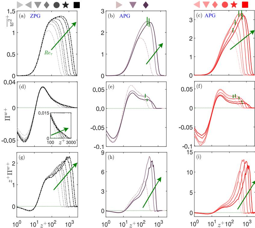
Figure 4: Wall-normal profiles for (a-c)  $\overline{w^2}^+$ , (d-f)  $\Pi^{w^+}$  and (g-i)  $z^+\Pi^{w^+}$  for ZPG (left column) and APG TBL cases. Symbols/colors correspond to the various cases defined in figure 1, with light to dark shading indicating increasing  $Re_\tau$ . Note the inconsistent range of ordinate. Vertical green lines indicate  $\overline{u^2}$  outer peak locations.
