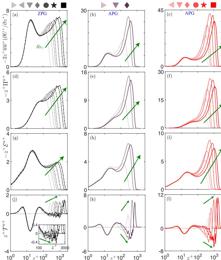
Figure 3: Wall-normal profiles for  $\overline{u^2}$ -transport terms pre-multiplied by  $z^+$ : (a-c)  $z^+ \mathcal{P}^{u+} \approx -2z^+ \overline{uw}^+ \partial U^+ / \partial z^+$ , (d-f)  $-z^+ \Pi^{u+}$ , (g-i)  $-z^+ \mathcal{E}^{u+}$  and (j-l)  $z^+ \mathcal{T}^{u+}$  for ZPG (left column) and APG TBL cases. Symbols/colors correspond to the various cases defined in figure 1, with light to dark shading indicating increasing  $Re_\tau$ . Note the inconsistent range of ordinate.
