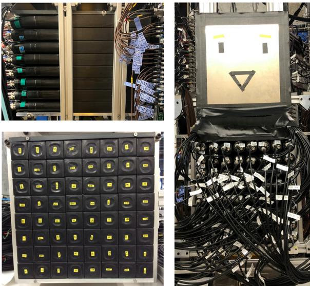
FIG. 6: Photographs of the calorimeter from three perspectives. **Top Left:** Side view from beam left. **Bottom Left:** Looking downstream towards the upstream face of the calorimeter. **Right:** Looking upstream at the full detector including the light-tight box on top of the crystals and the PMTs.
