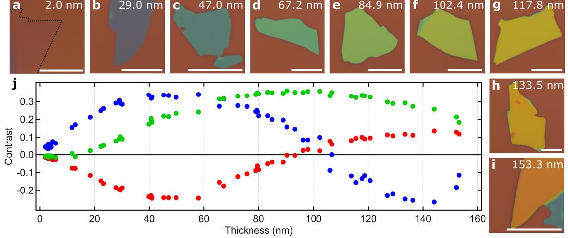
Figure 3: Optical microscope images of mechanically exfoliated biotite 1 flakes on an oxidized Si wafer (285 nm SiO<sub>2</sub>) in order of increasing thickness, ranging from (a) 2.0 nm (bilayer) to (i) 153.3 nm. The white scale bar in (a-i) is 20  $\mu$ m. (j) Optical contrast differences for the red, blue and green channels of all exfoliated flakes for the biotite 1 sample.
