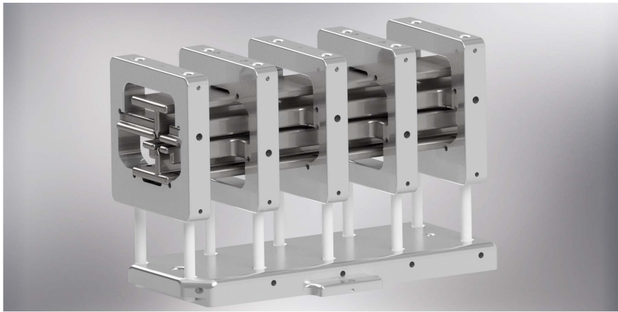
FIG. 9. Rendering of the merged guide assembly, showing the electrodes and their mounting brackets, ceramic support rods and base plate.
