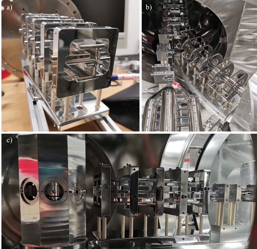
FIG. 10. Photos of the finished merged guide. (a) Photo from the exit hexapole, showing all six aluminum electrodes surrounding the beam axis. (b) Photo of the entire assembly, with a Stark decelerator feeding into a straight quadrupole followed by the straight arm of the merged guide. From the right, a curved hexapole guides the molecules to the entrance of the curved arm of the merged guide. (c) Photo of the last part of the assembly. From right to left, the straight quadrupole, merged guide and VMI lens.
