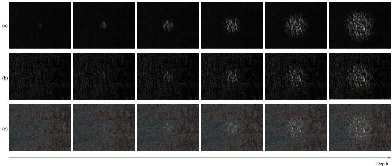
Fig. 8: Variation of interocular discrepancy maps with the increase of depth levels. Each row has the same distortion type and degree, but different depth levels. (a) JPEG compression; (b) Gaussian blur; (c) Additive white Gaussian noise.
