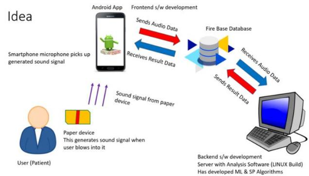
Fig. 3 Idea of the complete Spirometer system
