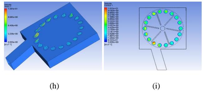
Fig. 2 Air flow simulations of Axial (a) - (e) and Tangential devices (f) - (i)
