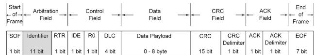
Fig. 1. Standard CAN frame format: 1-bit Start of Frame (SOF), 11-bit ID, 1-bit Remote Transmission Request (RTR), 1-bit Identifier Extension Bit (IDE), 1-bit Reverse R0, 4-bit Data Length Code (DLC), 0 to 8 byte data payload, 15-bit Cyclic Redundancy Check (CRC), 1-bit CRC delimiter, 1-bit Acknowledge (ACK), 1-bit ACK delimiter, and 7-bit End of Frame (EOF).
