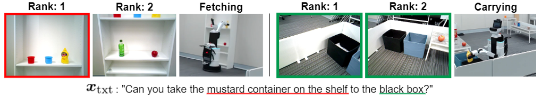
Figure 8. Qualitative results of the physical experiments. The target object images and receptacle images are framed in red and green, respectively. The words underlined in red and green indicate \mathbf{x}_{\text{targ}} and \mathbf{x}_{\text{rec}} , respectively.
