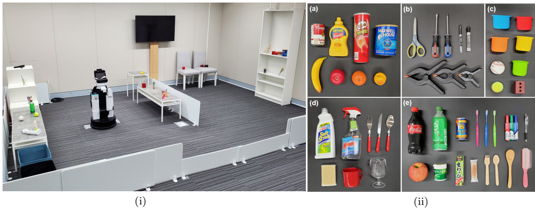
Figure 7. Experimental settings. (i) Domestic environment standardized in WRS2020RS [5]. (ii) Everyday objects used in the physical experiments. These objects are (a) ‘Food items,’ (b) ‘Tool items,’ (c) ‘Shape items,’ and (d) ‘Kitchen items’ from the YCB object set [50], and (e) general unseen objects.
