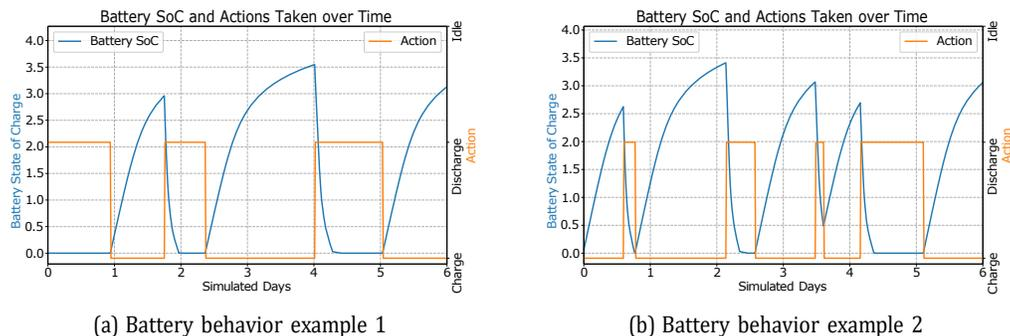
Figure 3: Battery State of Charge (SoC) and actions taken over time under two different random behaviors. The actions are labeled as Charge, Discharge, and Idle.
