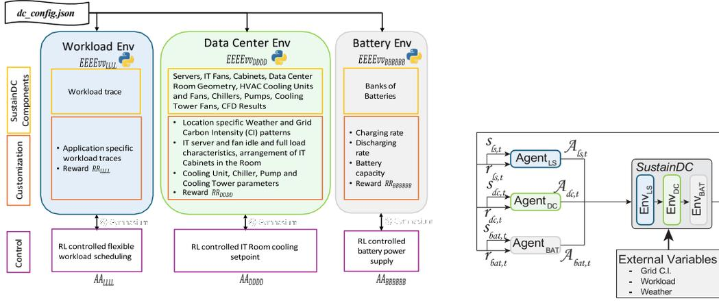
(a) High-level overview of SustainDC, showing the three main environments (*Workload Env*, *Data Center Env*, and *Battery Env*) along with their customizable components and control actions.
