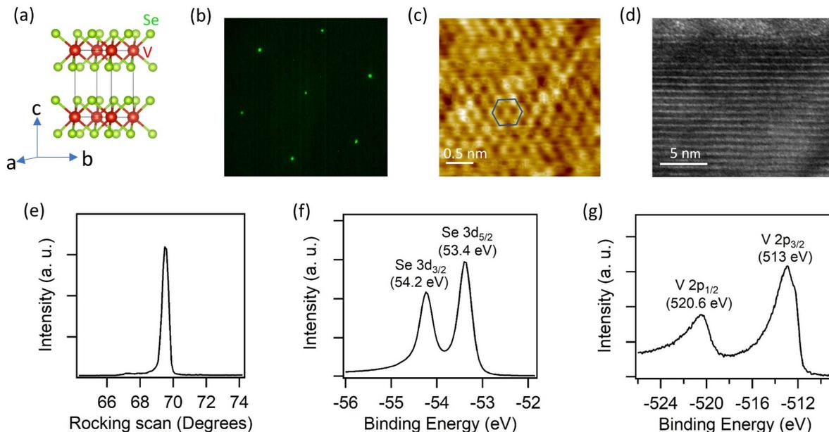
FIG. 1. (a) Ball-stick representation of 1T-VSe<sub>2</sub> crystal structure. (b-e) LEED pattern, STM image, HAADF-STEM cross-section image, and XRD pattern, respectively. (f-g) Se 3*d* and V 2*p* core levels spectra. All data were taken at room temperature except for the core levels recorded at 10 K. The blue hexagon in c represents the in plane unit cell. The STM image was recorded with a sample bias of 100 mV and set point of 1 nA.
