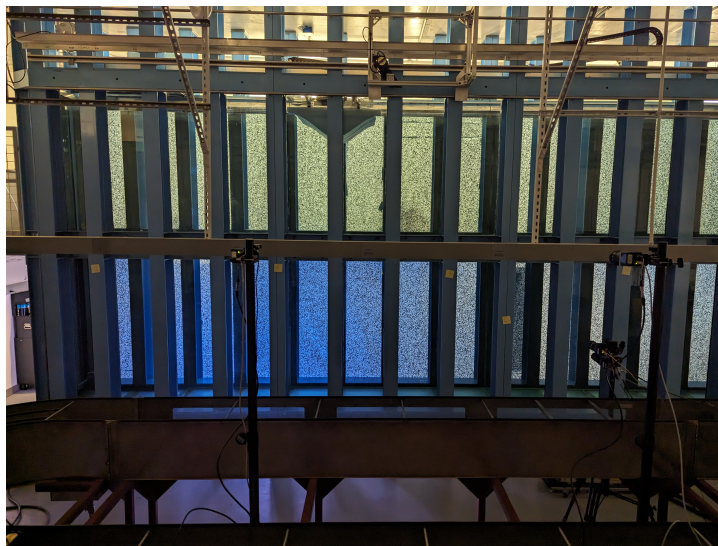
Figure 2: Photo of experimental setup showing random dot pattern paper on the far side of the tank, illuminated by lights.
