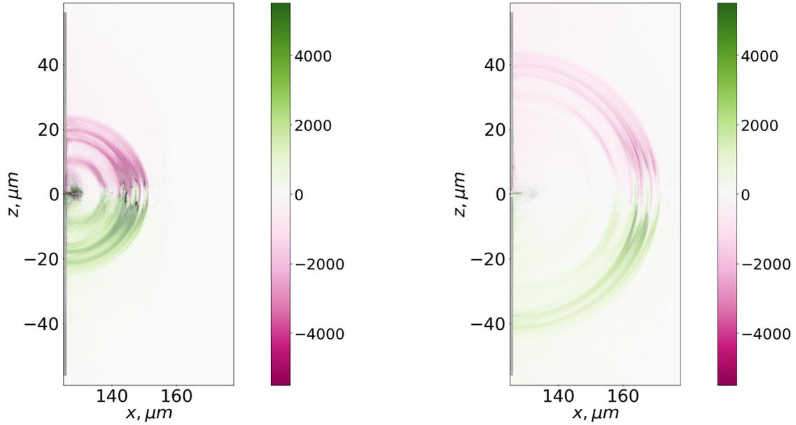
FIG. 3: The emitted electromagnetic field ( $B_y$  component) behind the plasma-vacuum interface from the PIC simulation for 10 fs laser pulse at two instants. The legend is given in T.
