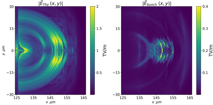
FIG. 6: Radiated (left panel) and intrinsic (right panel) electric fields of electron bunch for the case of 10 fs laser pulse with additional metal foil.
