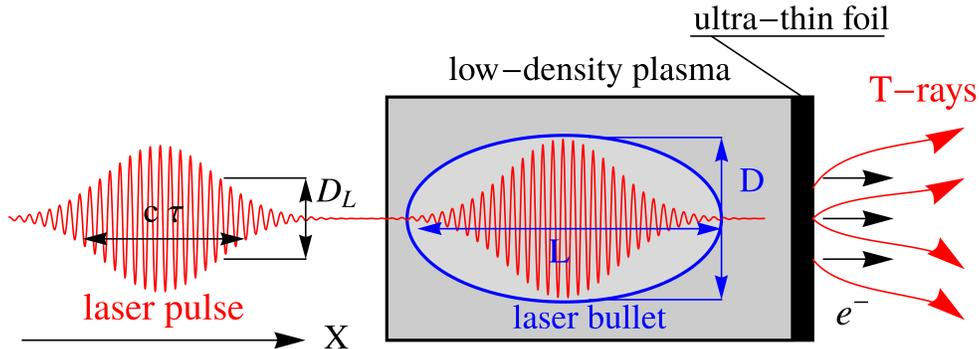
FIG. 1: Schematic illustration of the THz-generation scenario through CTR by the electrons based on the "laser bullet" RST regime.
