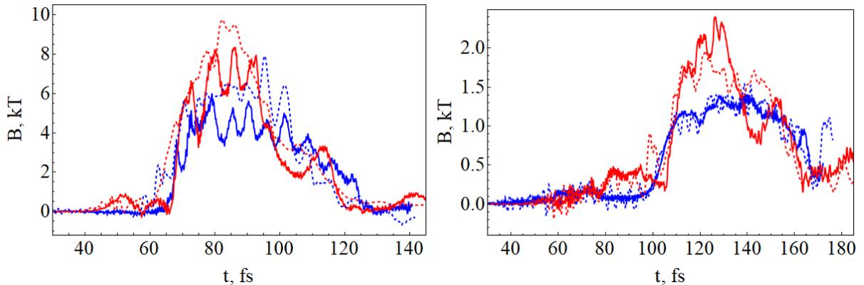
FIG. 4: Magnetic field component  $B_y$  behind the target at the distance of  $16 \mu\text{m}$ : (left) near the electron bunch,  $z = 5 \mu\text{m}$  and (right) closer to the periphery,  $z = 25 \mu\text{m}$ , for the 10 fs (dashed red) and 30 fs (dashed blue) laser pulses. The results for the case with additional foil are shown by the solid curves.
