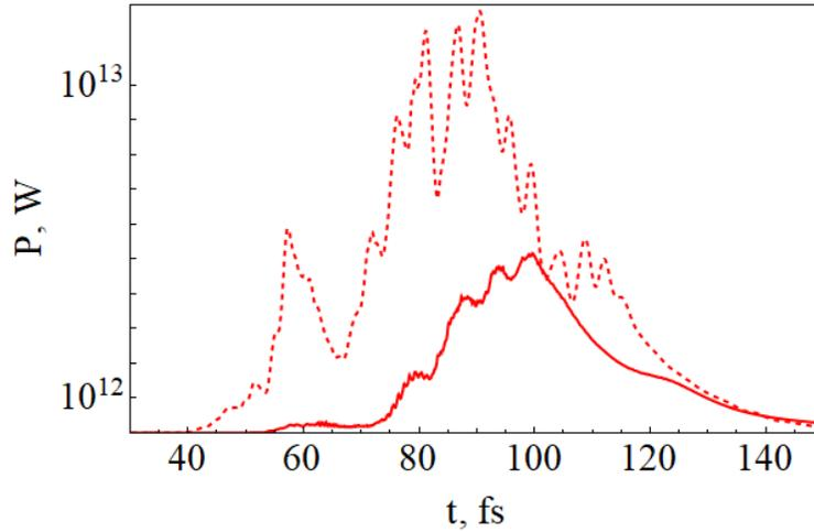
FIG. 7: Evolution of the radiated power at the surface with radius of  $16\mu\text{m}$  from target for the 10 fs laser pulse in the case with a foil at the back side (solid curve) and without a foil (dashed curve).
