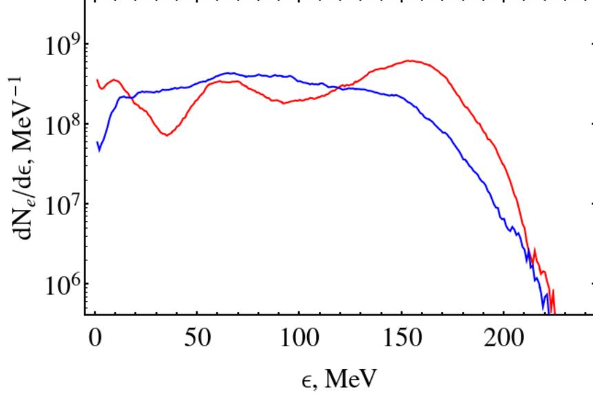
FIG. 2: Electron spectra generated in the RST regime by 30 fs (blue curve) and 10 fs (red curve) laser pulses.
