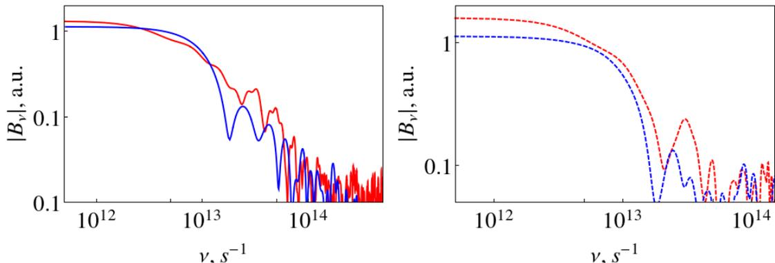
FIG. 5: Spectra of the CTR field at the distance of  $z = 16 \mu\text{m}$  with deviation  $z = 15 \mu\text{m}$  from the axis for the transparent plasma with an ultrathin foil at the target back side (left) and without foil (right side) for 10 fs laser pulse (red) and for 30 fs laser pulse (blue).
