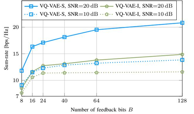
Fig. 6: The sum-rate over the number of feedback bits  $B$ , for a system with  $J = 8$  MTs,  $n_p = 8$  pilots, and  $\text{SNR} \in \{10 \text{ dB}, 20 \text{ dB}\}$ .
