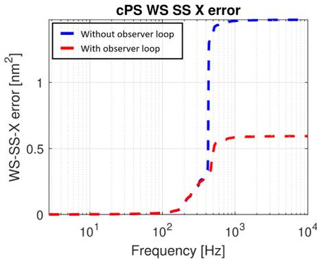
Figure 7: Cumulative power spectral density of the raw position tracking error in  $x$ -direction ( $u_{RB}^x \rightarrow y_{RB}^x$ ), where the blue graph corresponds to the cPS of the conventional rigid body control structure and the red graph denotes the cPS of the proposed control approach.
