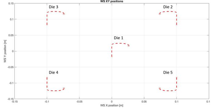
Figure 5: Five motion profiles that are considered to evaluate improvement of position tracking performance using the proposed control approach.
