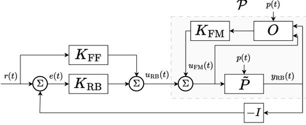
Figure 1: Proposed extension of the rigid-body control interconnection to allow for active regulation of position dependent flexible dynamics.
