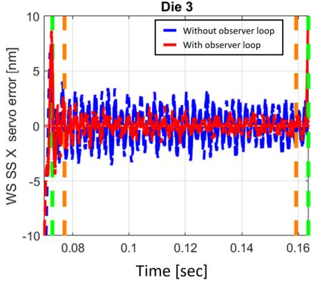
Figure 6: Raw position tracking error of Die 3, where the blue graph corresponds to the conventional rigid body control structure and the red graph corresponds to the proposed control approach. The green window indicates the constant velocity interval and the orange window indicates the exposure interval.
