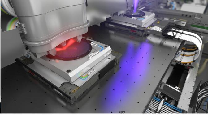
Figure 3: State-of-the-art EUV wafer stage system.
