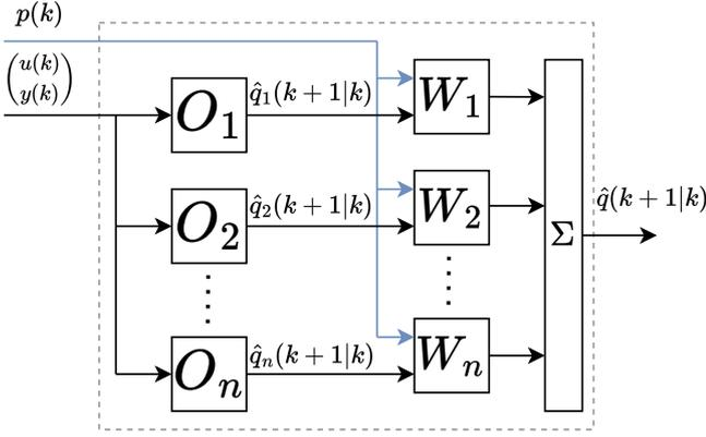
Figure 2: Block interconnection of proposed position dependent observer implementation for the estimation of a single position dependent flexible mode, where the modal states are approximated through a weighted sum of the outputs of the set of local observers  $\{O_i\}_{i=1}^n$ .
