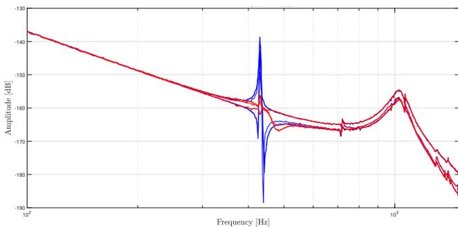
Figure 4: Local FRF measurements of the *equivalent mechanics*  $\mathcal{P}$  of the transfer in  $x$ -direction ( $u_{RB}^x \rightarrow y_{RB}^x$ ), where the blue graph corresponds to local FRF measurements of the conventional rigid body control loop. The red graph denotes to FRF measurements for which the proposed active damping loop is closed.
