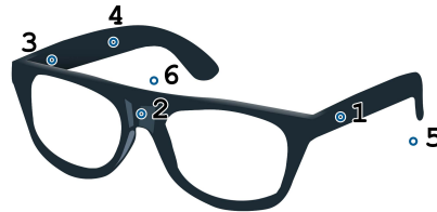
Fig. 9 An illustration of the microphone array mounted on a pair of glasses that was used in the listening experiment [58]. Only the microphones labeled 1-4 were used for performing the BSM reproduction.
