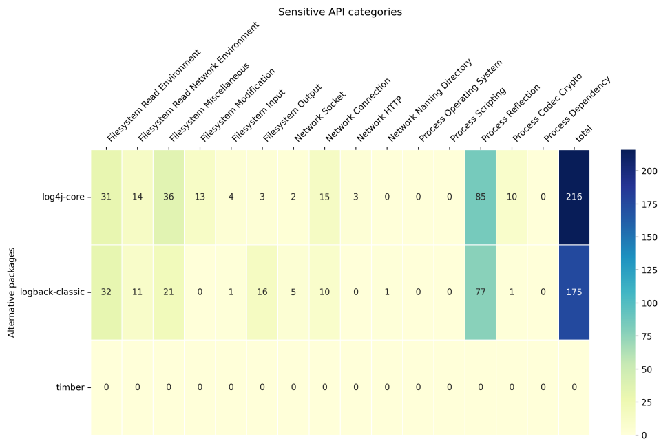
FIG. 6. Logging packages' security-sensitive API usage
