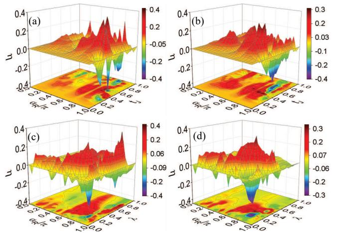
FIG. 3: The Josephson diode efficiency  $\eta$  for (a)  $N_x = 1$  and (b)  $N_x = 10$  in the  $(\alpha_R, t_J)$  space and for (c)  $N_x = 1$  and  $N_x = 10$  in the  $(\alpha_R, \lambda)$  space. For the width of the junctions, we have taken  $N_y = 15$ . In (a) and (b),  $\lambda$  is taken as 0.3; in (c) and (d),  $t_J$  is taken as 0.5.
