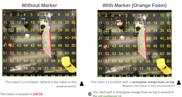
Fig. 6: Interpreting VLM Localization: We add numbers to the image taking inspiration from recent works [42], [43] to better interpret VLM localization. On the left image, note VLM prediction error in predicting the wrong cell, which is mitigated by adding an orange marker on the turtlebot.
