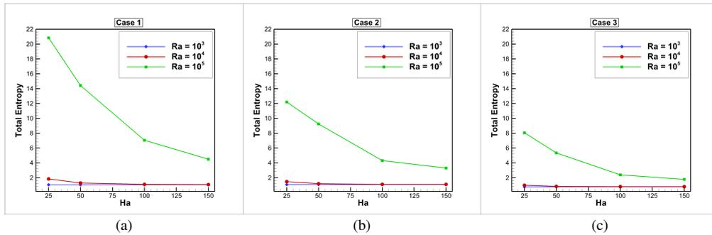
Figure 25: Influence of varying  $Ha$  and  $Ra$  on total entropy for (a) Case 1 (b) Case 2 (c) Case 3
