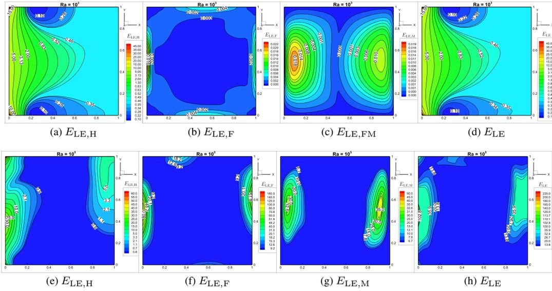
Figure 20: Case 2. Influence of  $Ra$  ((a-d)  $Ra = 10^3$ , (e-h)  $Ra = 10^5$ ) on entropy generation contours with fixed  $Ha = 25$
