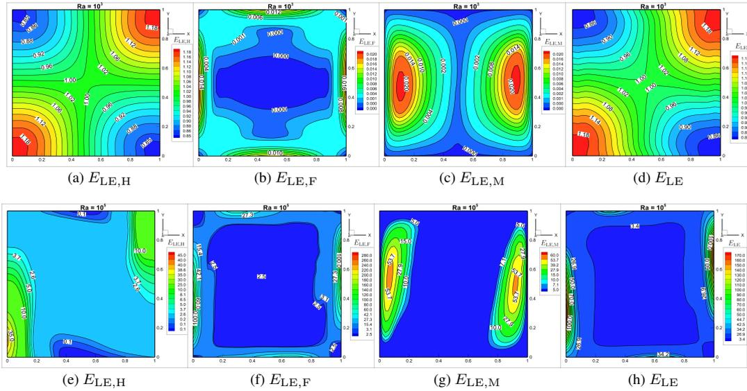
Figure 19: Case 1. Influence of  $Ra$  ((a-d)  $Ra = 10^3$ , (e-h)  $Ra = 10^5$ ) on entropy generation contours with fixed  $Ha = 25$
