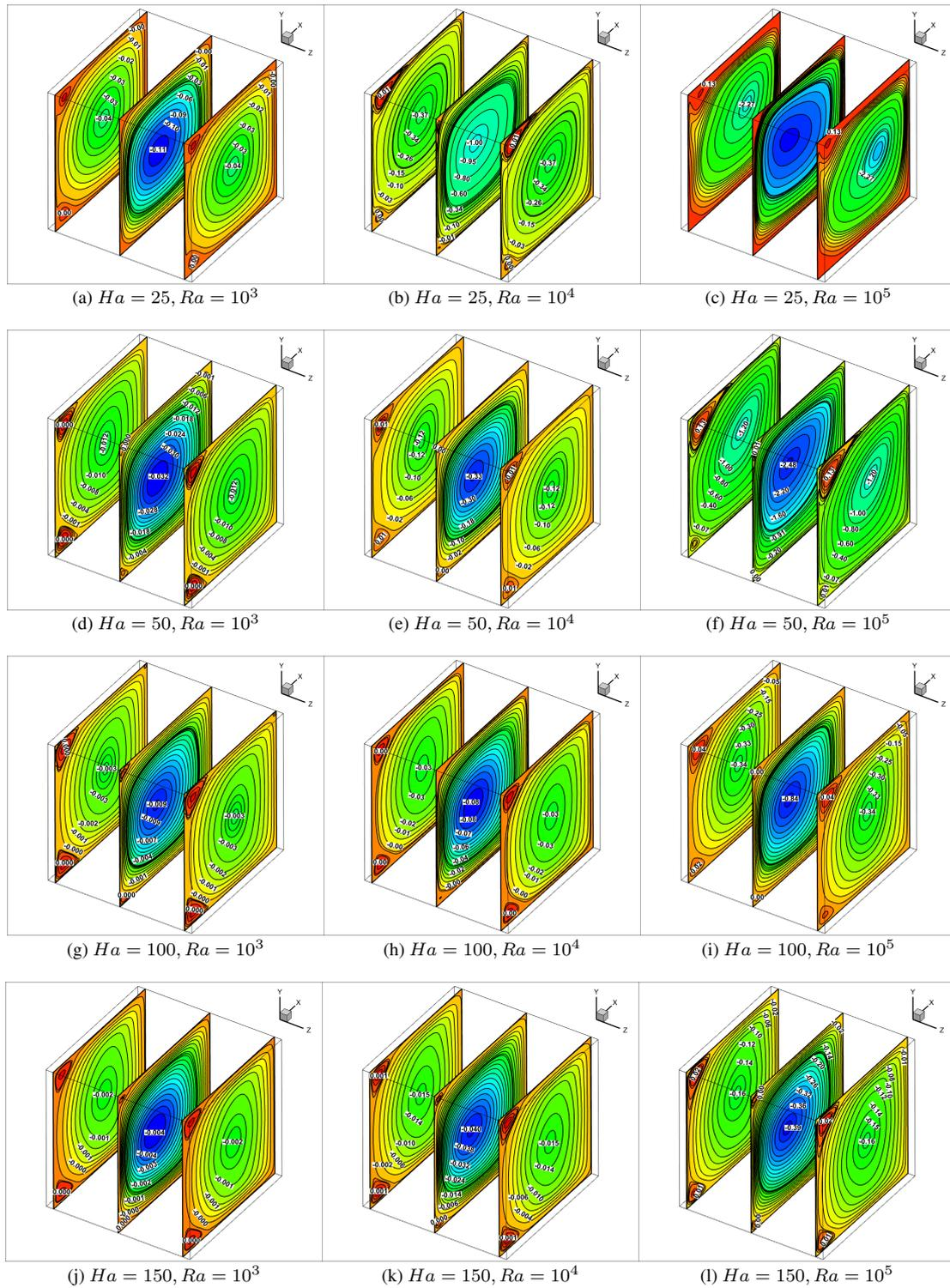
Figure 11: Case 3. Effect of different  $Ha$  (Column-wise) and  $Ra$  (Row-wise) on streamlines pattern at different  $xy$  planes ( $z = 0.05, z = 0.5, z = 0.95$ ) with fixed  $Pr = 0.065$
