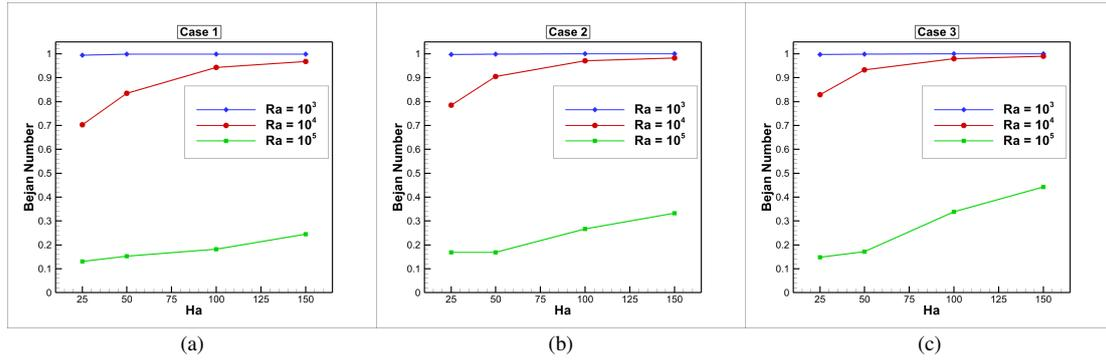
Figure 26: Influence of different  $Ha$  and  $Ra$  on Bejan number ( $Be$ ) for (a) Case 1 (b) Case 2 (c) Case 3
