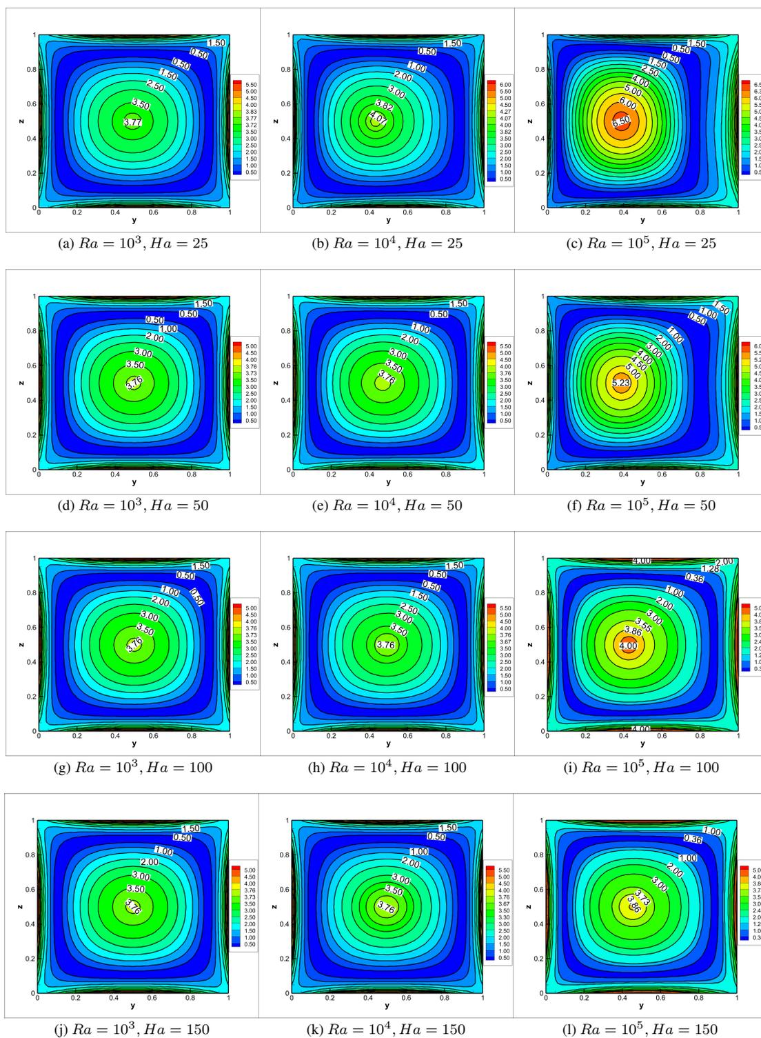
Figure 16: Case 3.  $Nu_L$  contours on the left ( $x = 0$ ) heated wall of the cubic cavity
