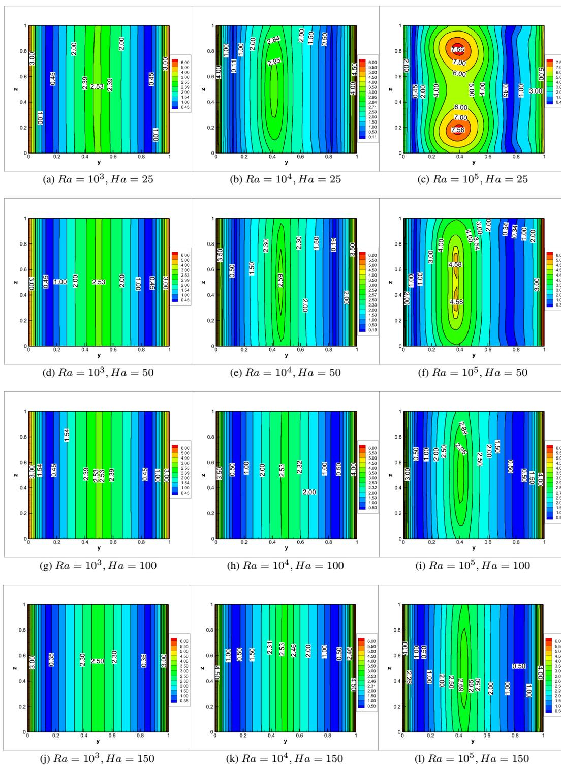
Figure 15: Case 2.  $Nu_L$  contours on the left ( $x = 0$ ) heated wall of the cubic cavity
