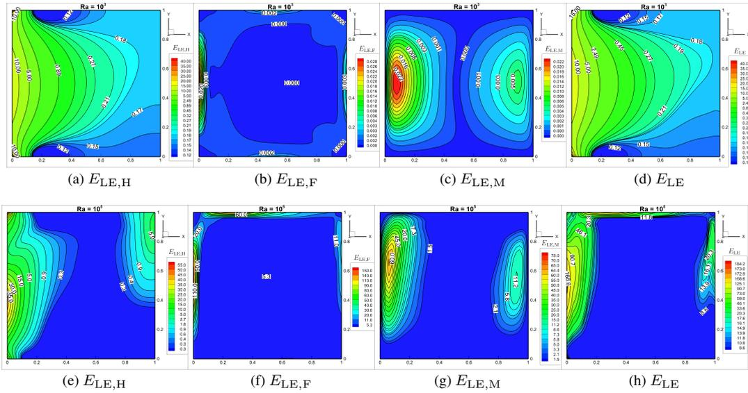
Figure 21: Case 3. Influence of  $Ra$  ((a-d)  $Ra = 10^3$ , (e-h)  $Ra = 10^5$ ) on entropy generation contours with fixed  $Ha = 25$
