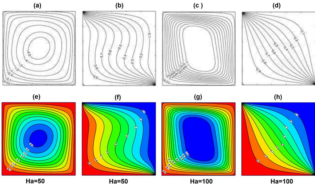
Figure 3: Comparison of stream-function and isotherm contours (at  $Ra = 10^5$ ) between (a-d) existing [29] and (e-h) present computed results
