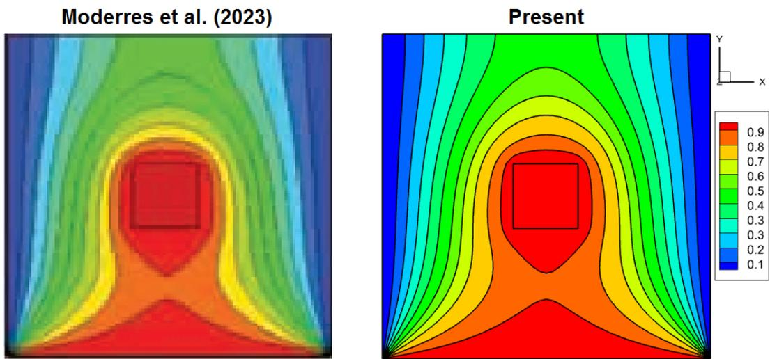
Figure 4: Comparison of Isotherms (at  $Ra = 10^3$ ,  $Ha = 90$ ) for natural convection on symmetry plane ( $z = 0.5$ ): Moderres et al. (2023) [44] vs. present result
