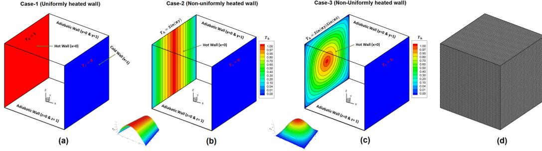
Figure 1: (a-c) Schematic view of the problem for three different cases (d) Visualization of the grids with  $51 \times 51 \times 51$  grid size.
