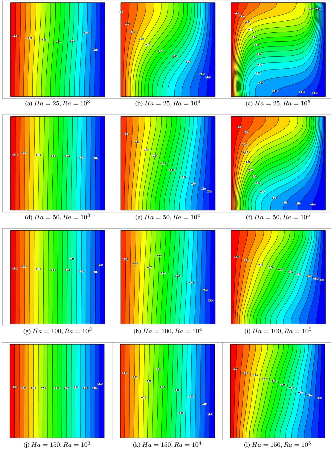
Figure 7: Case 1. Effect of different  $Ha$  (Column-wise) and  $Ra$  (Row-wise) on isotherm contours (at  $z = 0.5$  plane) at a fixed  $Pr = 0.065$
