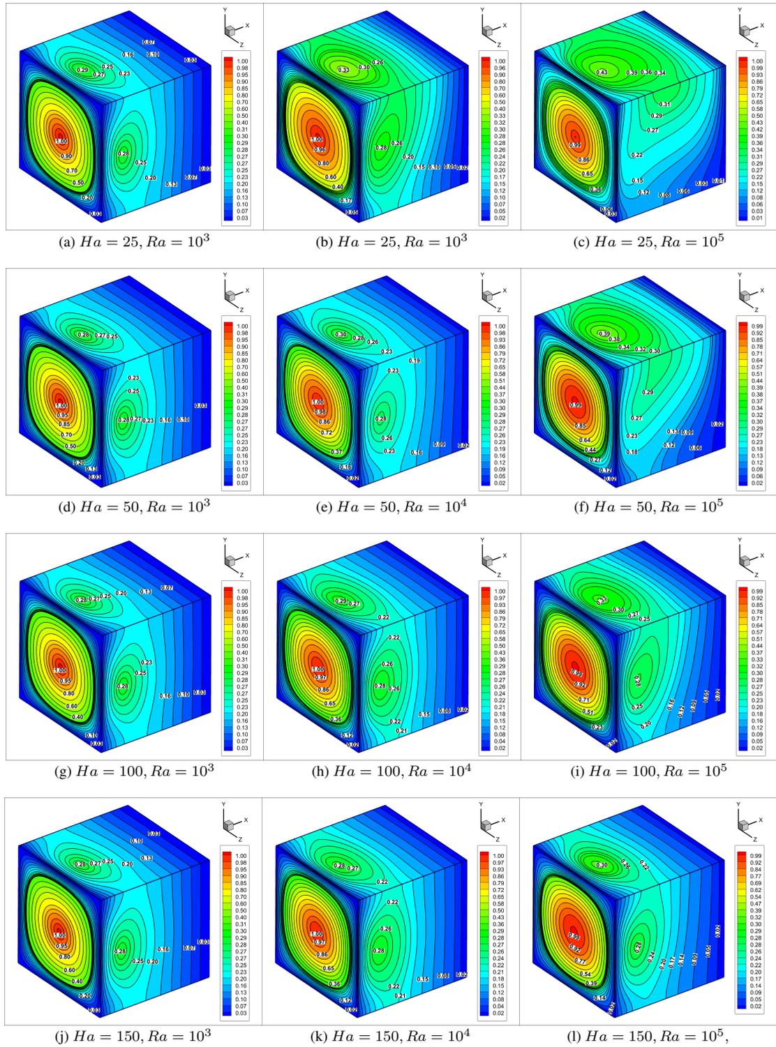
Figure 12: Case 3. Effect of different  $Ha$  (Column-wise) and  $Ra$  (Row-wise) on isotherm contours at a fixed  $Pr = 0.065$
