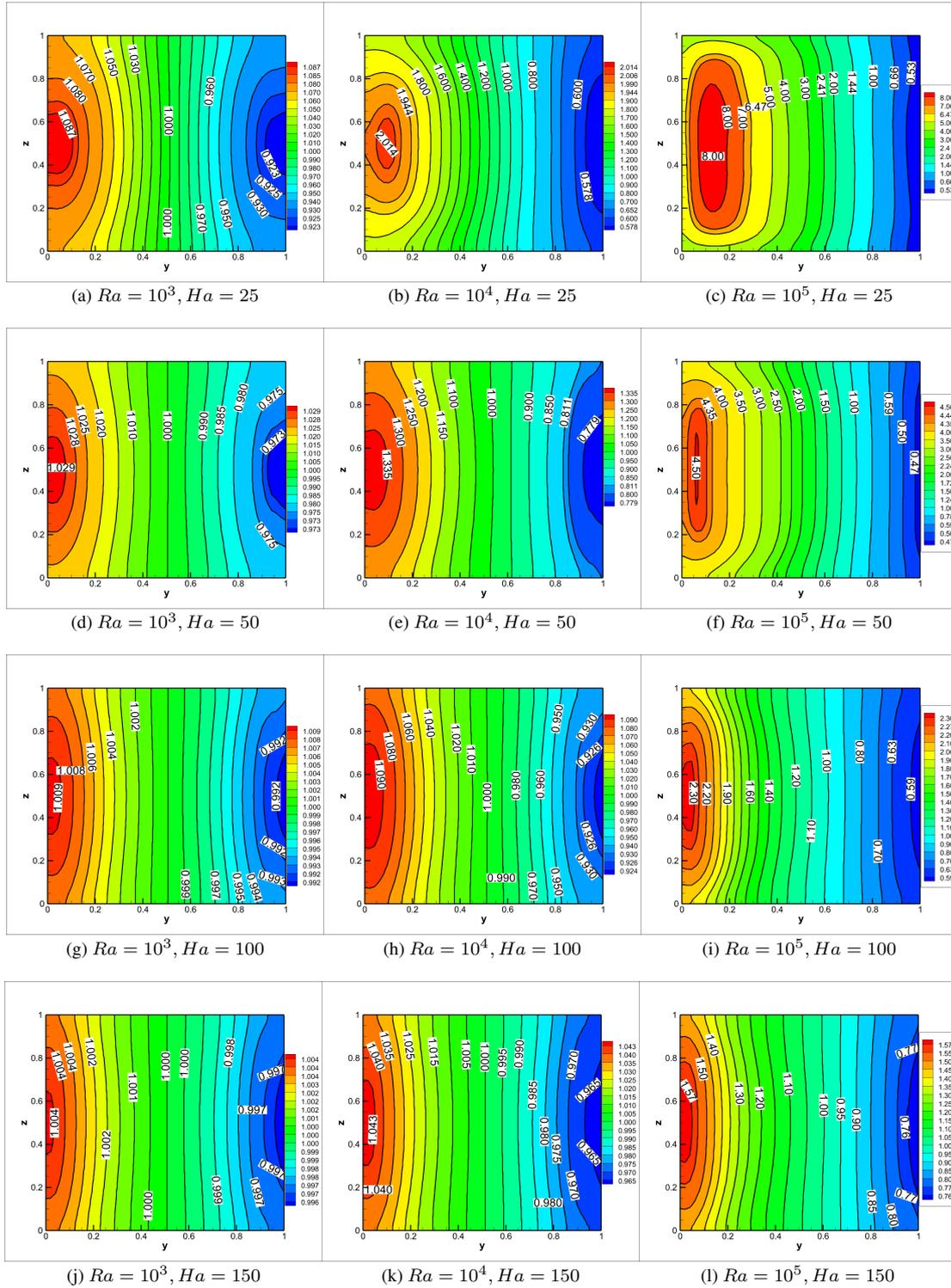
Figure 14: Case 1.  $Nu_L$  contours on the left ( $x = 0$ ) heated wall of the cubic cavity
