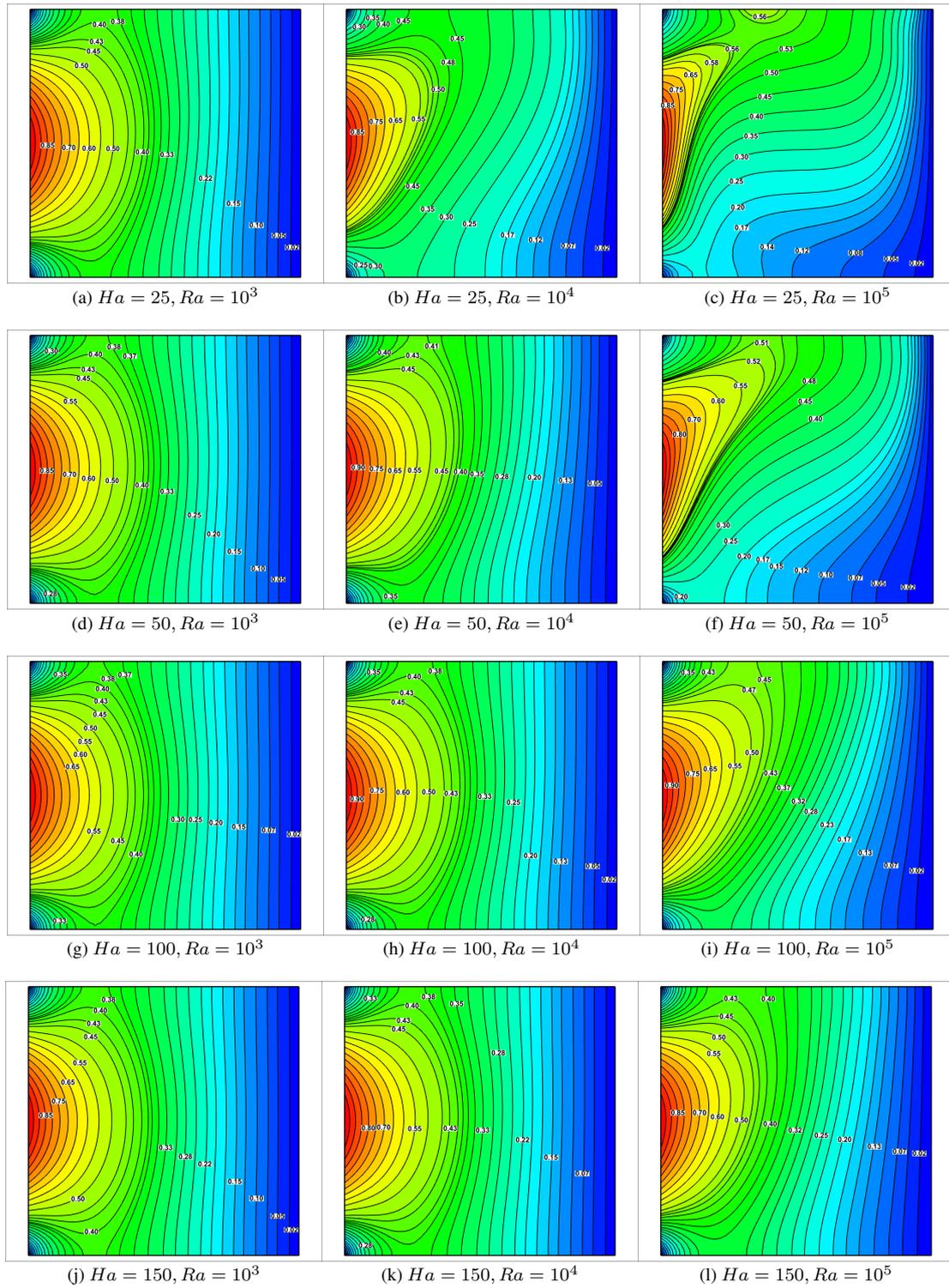
Figure 10: Case 2. Effect of different  $Ha$  (Column-wise) and  $Ra$  (Row-wise) on isotherm contours (at  $z = 0.5$  plane) at a fixed  $Pr = 0.065$
