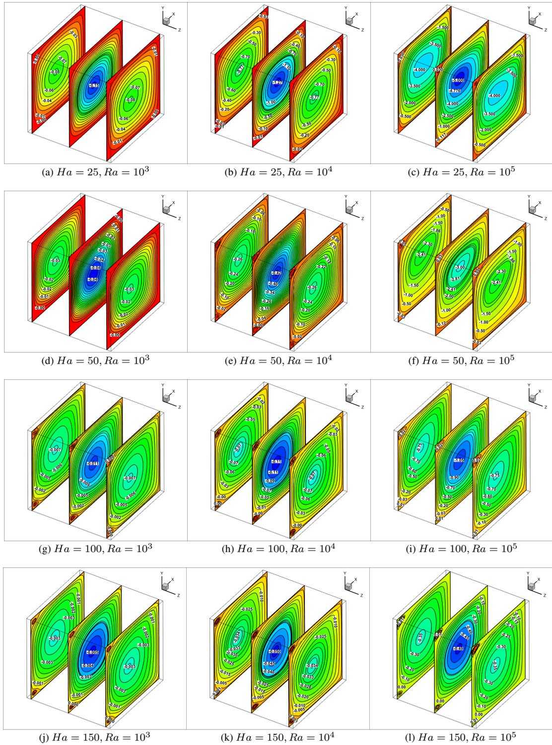
Figure 8: Case 2. Effect of different  $Ha$  (Column-wise) and  $Ra$  (Row-wise) on streamlines pattern at different  $xy$  planes ( $z = 0.05, z = 0.5, z = 0.95$ ) with fixed  $Pr = 0.065$
