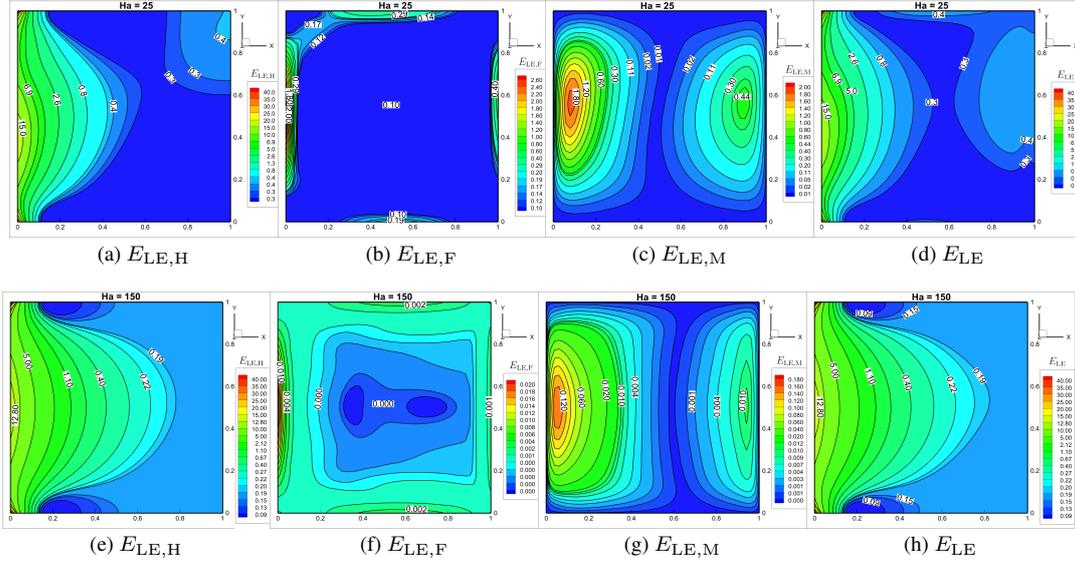
Figure 24: Case 3. Influence of different  $Ha$  ((a-d)  $Ha = 25$ , (e-h)  $Ha = 150$ ) on entropy generation contours with fixed  $Ra = 10^4$
