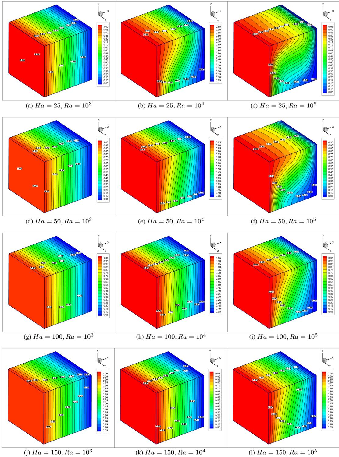
Figure 6: Case 1. Effect of different  $Ha$  (Column-wise) and  $Ra$  (Row-wise) on isotherm contours at a fixed  $Pr = 0.065$
