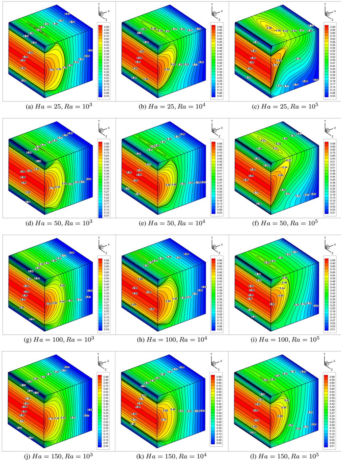
Figure 9: Case 2. Effect of different  $Ha$  (Column-wise) and  $Ra$  (Row-wise) on isotherm contours at a fixed  $Pr = 0.065$
