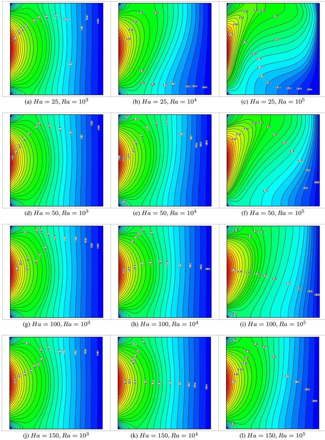
Figure 13: Case 3. Effect of different  $Ha$  (Column-wise) and  $Ra$  (Row-wise) on isotherm contours (at  $z = 0.5$  plane) at a fixed  $Pr = 0.065$
