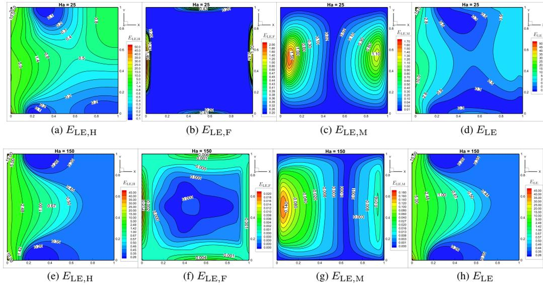
Figure 23: Case 2. Influence of different  $Ha$  ((a-d)  $Ha = 25$ , (e-h)  $Ha = 150$ ) on entropy generation contours with fixed  $Ra = 10^4$
