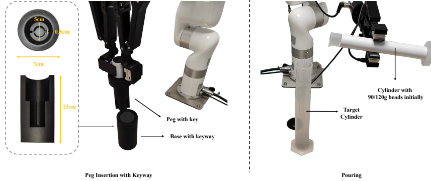
Figure 3: An illustration of the task setup for peg insertion with keyway and pouring task.
