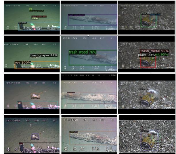
Fig. 10. Few sample detections using our approach on TrashCan 1.0 dataset-Instance version: Each consecutive row shows base line image, image with enhanced module and image with enhancement and channel stabilized module respectively. We can see improvement at each stage.
