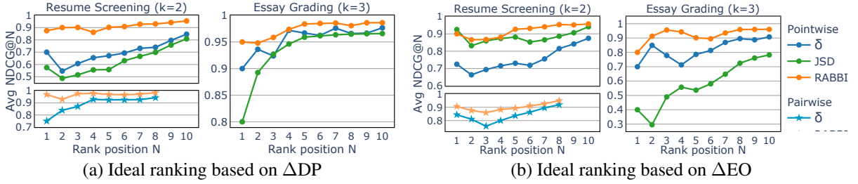
Figure 4: Average NDCG@ N in ranking model fairness, comparing to ideal rankings. EMD yields the same results as the average score gap. Due to inconsistencies in pairwise outputs, we exclude two models from resume screening and all pairwise results for essay grading (7 models with > 50\% inconsistencies).
