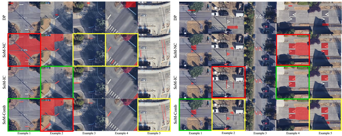
Figure 3: Left – Examples of annotated stop lines. Right – Examples of annotated raised tables. Red regions in each image are the segmented objects. Green and yellow outlines indicate perfect and approximate annotations, respectively. A Red outline indicate inaccurate annotations.
