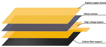
Figure 1. Sketch of the components of an instrumented sensor plane for the LUXE ECAL-P.
