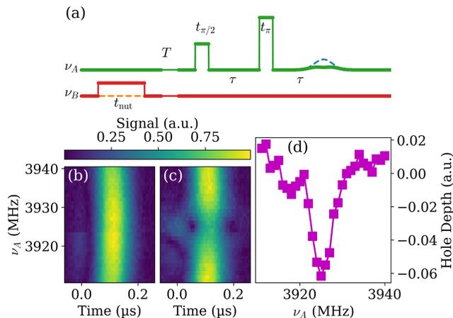
FIG. 6. Demonstration of a two-tone hole-burning experiment. (a) Pulse sequence schematic for the experiment, showing the nutation pulse at  $\nu_B$  and the Hahn echo sequence at  $\nu_A$ . The time between the nutation pulse and the first Hahn echo pulse is truncated for clarity. (b,c) Background-subtracted echo data without (b) and with (c) the nutation pulse, using the parameters given in the text. (d) Depth of the hole as a function of frequency. The hole width is  $5.6 \pm 0.7$  MHz.
