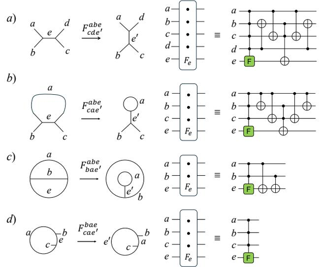
Figure 9. The  $F$ -move and its circuit implementations. (a) The general form of  $F$ -move with five inputs. (b) A simplified  $F$ -move with four inputs. (c) A further simplified  $F$ -move for three inputs. (d) A special case of  $F$ -move with four inputs.
