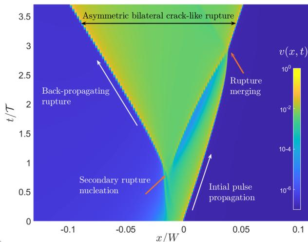
FIG. 5. Results of the same computation as in Fig. 4c-d, presented here in a space-time  $x-t$  plot. The slip velocity field  $v(x, t)$  (in units of m/s, as in Fig. 4c) is plotted on a logarithmic scale, see color legend on the right.  $x$  is normalized by the fault size  $W$  and  $t$  by  $\mathcal{T} \equiv L^{(0)}/c^{(0)}$ . All dynamical events and various rupture propagation modes are marked, see text for additional discussion.
