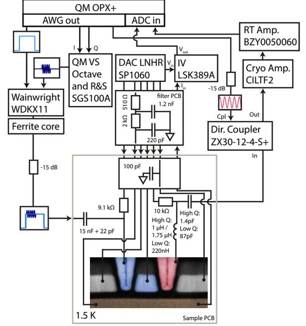
FIG. 6. Full experimental setup
