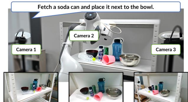
**Figure 1.** An example problem. We use three RGB cameras, one of which is attached to the end-effector, and the rest are fixed facing the cabinet. Multiple objects including shiny and transparent objects are on the shelf. The robot must ground the language command to objects and plan a collision-free pick-and-place motion to achieve the goal.
