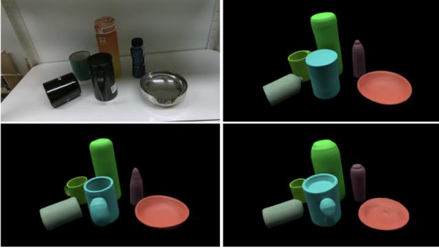
**Figure 9.** Visualization of stochastic outputs from the diffusion estimator of DEF-oriCORN. The upper left figure displays the real-world configuration, while the three other figures show the predictions. The samples capture different details of features that are not clearly distinguishable from the image, such as the handle of the black cup and the shape of the blue cup.
