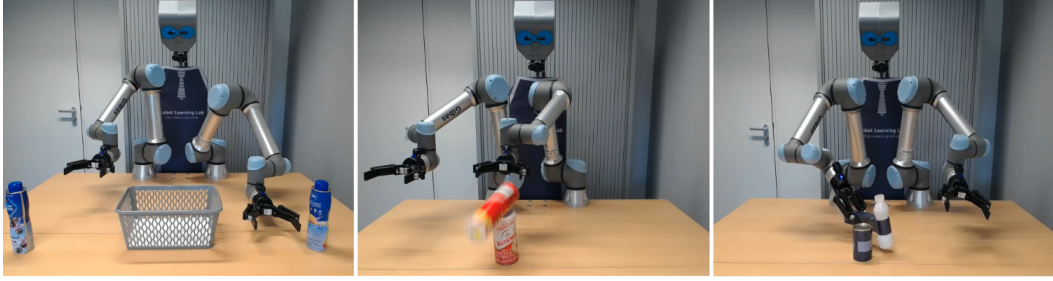
Figure 21: Various failure cases observed during the real robot experiments: (left) The robot fails to accurately grasp and place the bottles into the basket, likely due to errors in trajectory prediction. (center) The robot is unable to stack objects stably, with the objects either toppling over or not aligning correctly. This can be attributed to differences in the control systems between simulation and reality, as well as potential errors in trajectory predictions. (right) The robot fails to hit the target object during the hammering task. This failure can be caused by open-loop control limitations, differences in objects' shape, and errors in the predicted trajectories.
