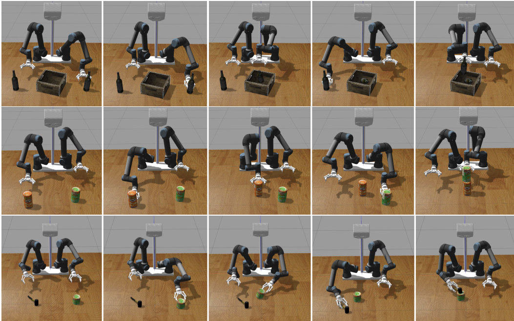
Figure 14: The images illustrate the step-by-step process of the robot as it performs the task of ( top-row ) collecting bottles, ( second-row ) stacking objects, ( lower-row ) hammering. This sequence demonstrates the robot’s ability to predict a sequence of subtasks and follow a predicted trajectory to complete the stacking task successfully.
