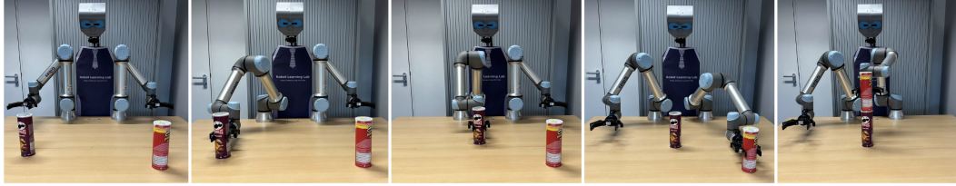
Figure 9: Sequence of snapshots demonstrating the stacking objects task performed by the real robot.
