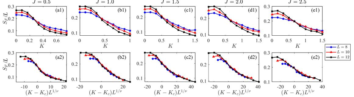
FIG. 6. (Color online) Finite-size scaling of  $S_F$  to determine the critical points  $K_c$ . The lower column shows  $S_F$  after the data collapse for  $J = \{0.5, 1.0, 1.5, 2.0, 2.5\}$  with  $K_c \approx \{0.28, 0.42, 0.51, 0.60, 0.70\}$  and critical exponent  $\nu \approx 0.65$  in (a-e), respectively.
