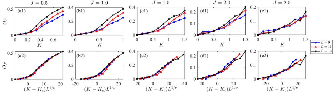
FIG. 5. (Color online) Finite-size scaling of  $O_F$  to determine the critical points  $K_c$ . The lower column shows  $O_F$  after the data collapse for  $J = \{0.5, 1.0, 1.5, 2.0, 2.5\}$  with  $K_c \approx \{0.2, 0.38, 0.52, 0.62, 0.75\}$  and critical exponent  $\nu \approx 0.70$  in (a-e), respectively.
