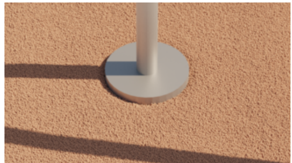
Fig. 5: Screenshot of the plate sinkage test with 0.2 m radius plate. Animation of the plate sinkage test simulation is provided in the supplementary materials.
