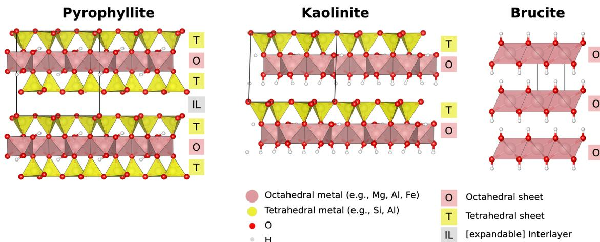
Figure 2: View onto three example representative clays: 2:1 pyrophyllite, 1:1 kaolinite and anionic clay brucite. The unit cell is shown in black, T sheet in yellow, O sheet in pink, and interlayer (IL) space marked in blue.
