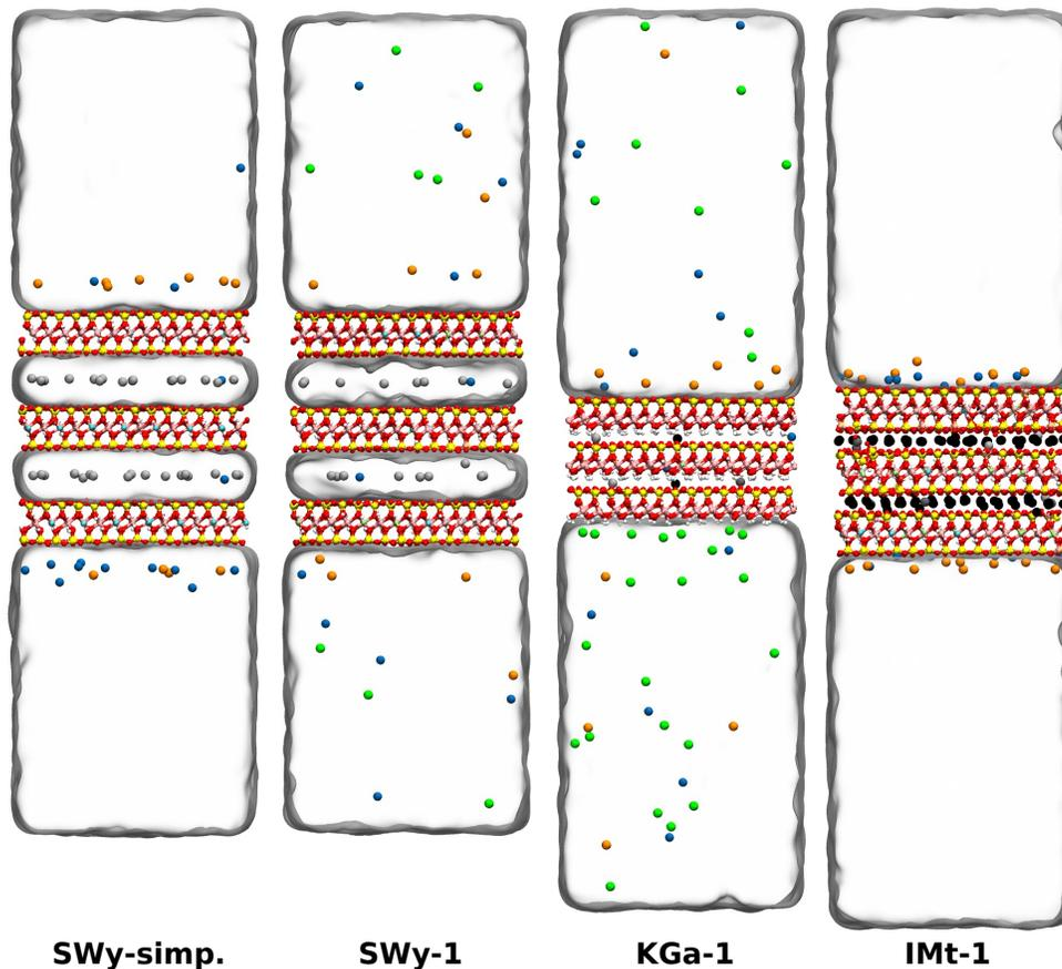
Figure 5: Side view of the four systems produced with *ClayCode*. Clay layers in the middle, water is represented as transparent surfaces and ionic species are shown as spheres of different colour.
