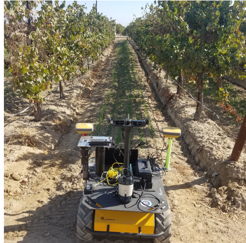
Fig. 1: Our robot has been retrofit with a soil moisture sensor that can be inserted in the soil to collect data at preassigned locations, or at locations decided by the robot on-the-fly (the soil moisture probe is visible on the left).
