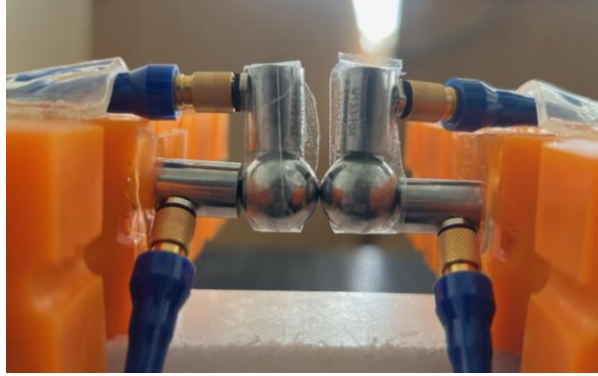
Figure A1: Experimental setup of the nonlinear granular network. One of the granules is driven by an ultrasonic transducer. Meanwhile, the lateral transducers record the responses of the vibrating granules.
