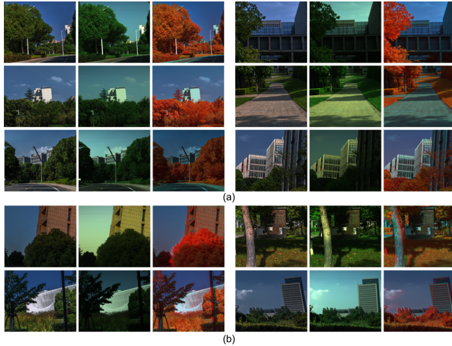
Fig. 3: We substitute the R channel in the smartphone-captured RGB image with the shading image, which allows for a visual evaluation of the image registration quality. In each sample, the first column is the smartphone-captured RGB image, the second column is the pseudo-RGB image from the hyperspectral data, the third column is the fused image which replaces the R channel with the shading image. (a) Samples in our Mobile-Spec dataset demonstrate high alignment accuracy. (b) Samples that exhibit artifacts and misalignments are discarded in the dataset filtering procedure.
