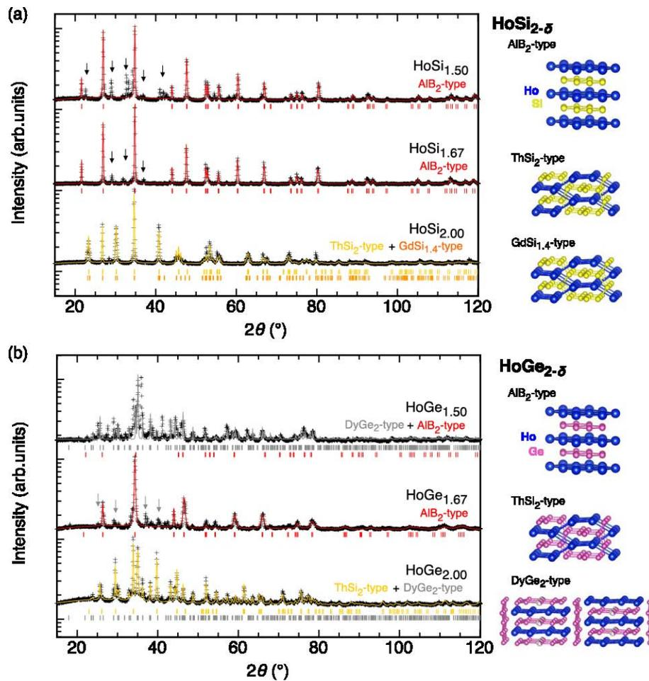
Figure 2: Powder x-ray diffraction patterns and their fitting. (a)  $\text{HoSi}_{2-\delta}$  and (b)  $\text{HoGe}_{2-\delta}$ . Corresponding crystal images are shown in the right panel. Additional peaks pointed by arrows are from unknown phases.
