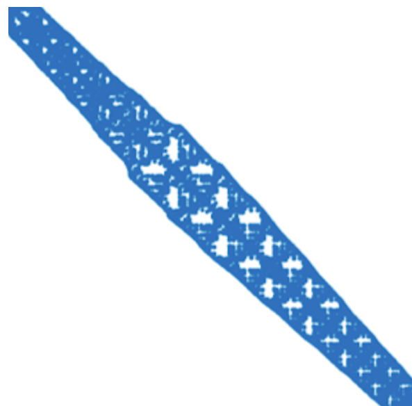
Figure 8. A closer look to general pattern of the band matrix Audikw_1 after RCM transformation. We split either lower or upper half of such band structure into three parts. The main diagonal is the dense and smallest split. The middle part contains majority of the data in the entire matrix, but it also has a very sparse structure. Middle split mostly covers data in non-racing regions under our partitioning approach (See yellow squares in Figure 2, explained in Part 3.) The distance from main diagonal to outer split is determined with a user specified bandwidth. This is to provide flexibility to achievable performance in cases where the sparsity structure and band size of the band matrix is well predicted.
