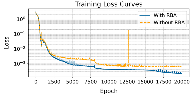
Fig. 5. Training loss of a PIKAN for the Allen-Cahn equation with (blue, solid line) and without (orange, dashed line) RBA.
