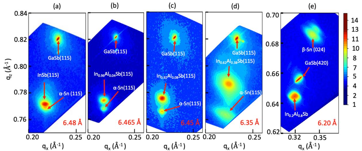
Figure 2. RSM scans of samples with different buffer layer lattice constants. RSM images for samples of (a) 6.48 Å, (b) 6.465 Å, (c) 6.45 Å, and (d) 6.35 Å with  $\alpha$ -Sn phase show strained thin films except for 6.35 Å sample, (e) RSM shows relaxed thin films for  $\beta$ -Sn phase in sample 6.20 Å.
