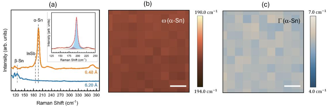
Figure 4. (a) Representative Raman spectra of  $\alpha$ -Sn (top, 6.48 Å) and  $\beta$ -Sn (bottom, 6.20 Å). The inset shows a fitted result of the Raman spectrum of  $\alpha$ -Sn, showing deconvoluted individual components of the 150, 187, 197, and 230  $\text{cm}^{-1}$  modes. Spatial variations in (b) peak frequencies and (c) spectral widths of the optical phonon of  $\alpha$ -Sn. The scale bars are 2  $\mu\text{m}$ .
