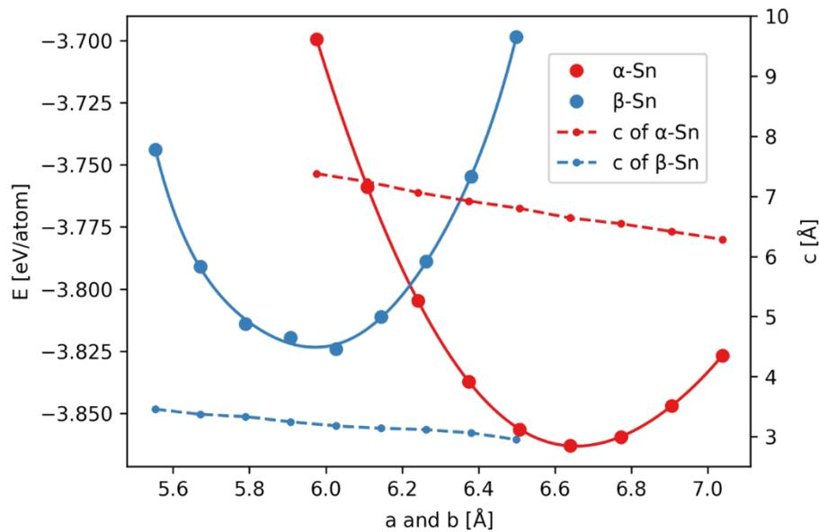
Figure 7. Total energies of  $\alpha$ -Sn and  $\beta$ -Sn with different lattice parameters,  $a$  and  $b$ . The lattice parameter  $c$  was optimized for the given  $a$  and  $b$ . Here the total energy is divided by the number of atoms in the unit cell considered in the calculations.
