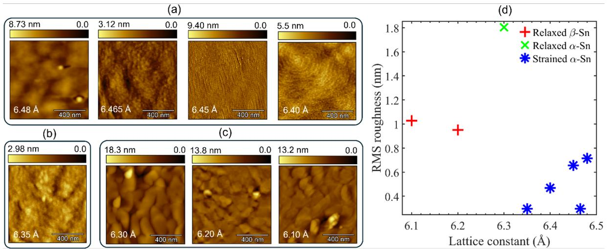
Figure 3. AFM images depicting the surface morphology of (a) strained  $\alpha$ -Sn, (b) relaxed  $\alpha$ -Sn, and (c) relaxed  $\beta$ -Sn phases of the samples. (d) RMS roughness of the samples as a function of buffer layer lattice constant, for a surface area of  $1\ \mu\text{m} \times 1\ \mu\text{m}$ .
