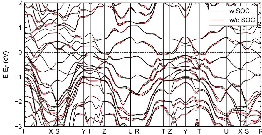
Figure 3: Band structure of the HP-II AFM1 structure at 12 GPa around the Fermi level, with and without Spin Orbit Coupling (SOC).
