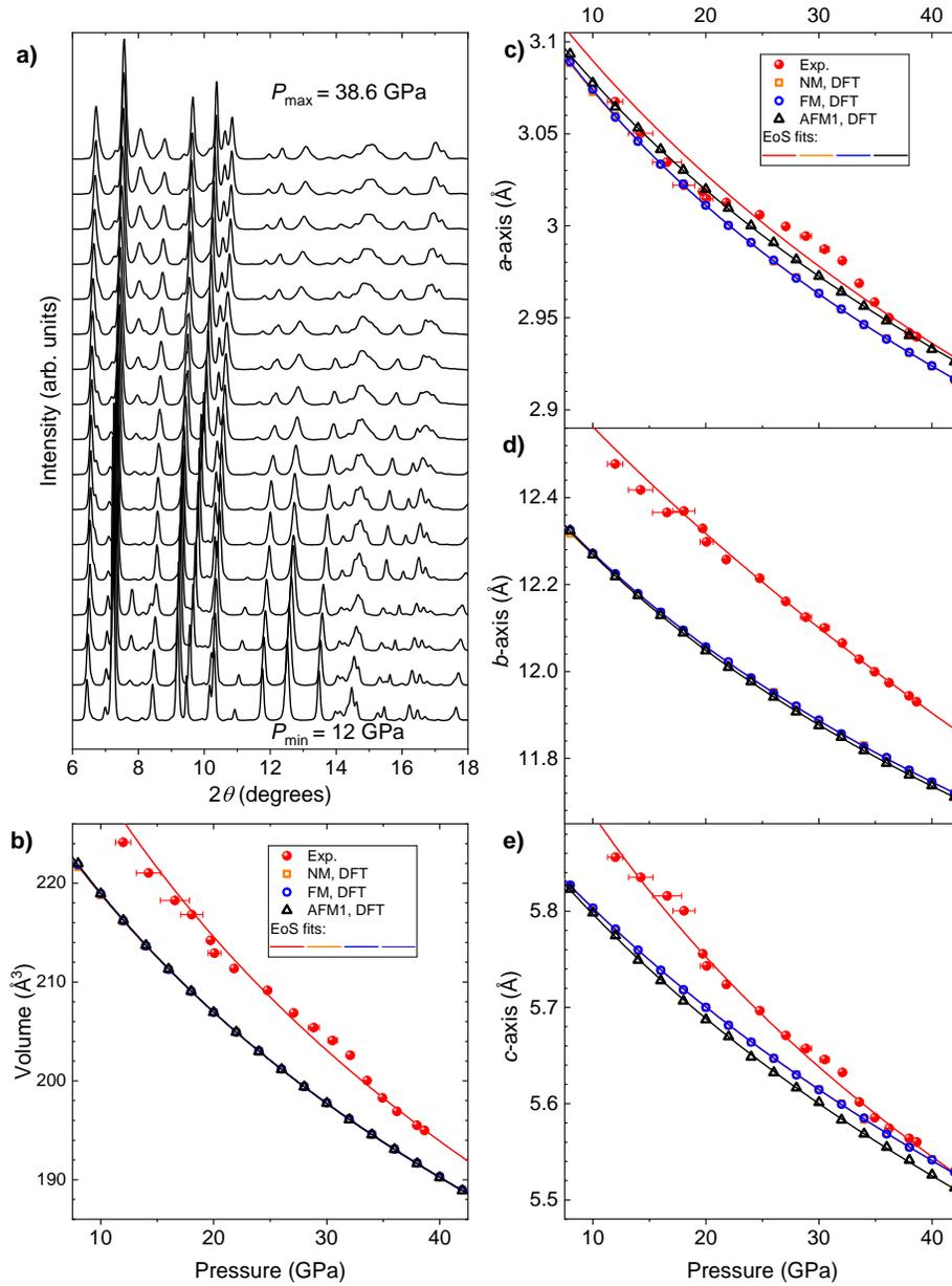
Figure 5: a) Background subtracted waterfall plot of the diffractograms for the HP-II phase. b-e) Experimental and calculated unit cell parameters for the HP-II structure.
