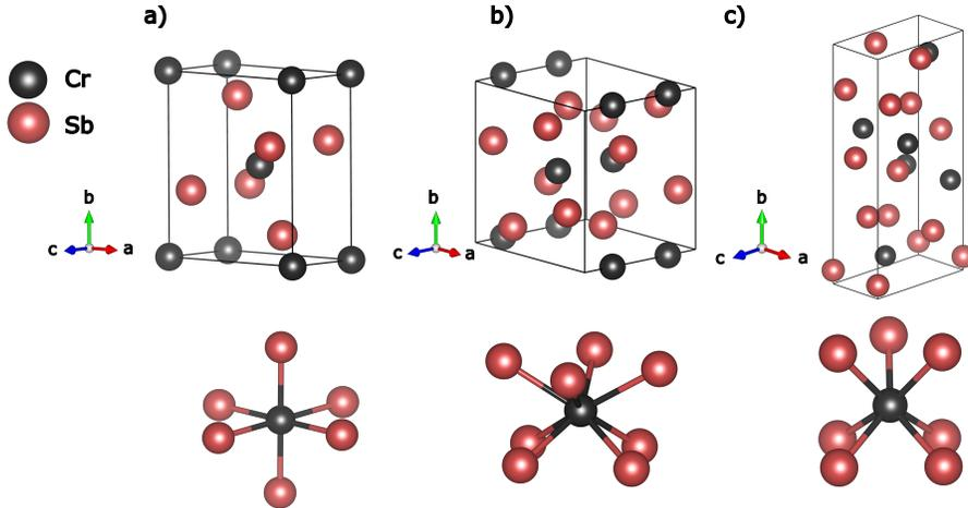
Figure 1: Crystal structure and Cr coordination of the different high-pressure polymorphs of CrSb<sub>2</sub>: **a)** Marcasite, **b)** CuAl<sub>2</sub>-type (HP-I) and **c)** MoP<sub>2</sub>-type (HP-II).
