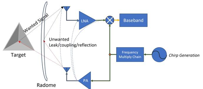
Fig. 1: Simplified FMCW radar architecture and self-interference paths.
