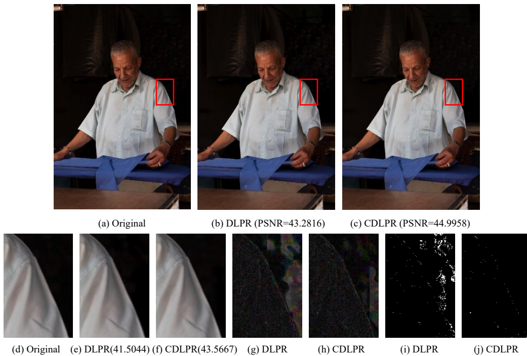
Figure 10. Experimental results of DLPR and CDLPR with maximum PSNR increment on CLIC2021 test image dataset.
