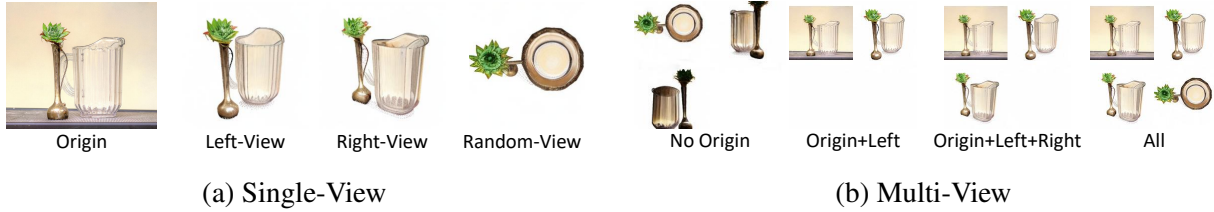
Figure 2: Single-view images were generated using Zero-1-to-3 to produce left-view, right-view, and random-view images. Multi-view images were created by combining these different single-view images in various configurations.
