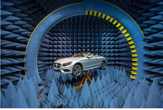
Fig. 1. Virtual Road – Simulation and Test Area (VISTA) at the Thuringian Center of Innovation in Mobility (ThIMo), without the BIRA bistatic measurement system installed. A passenger car is placed on the turntable (hidden under pyramidal absorbers) and elevated to the focal point of the antenna arch, enabling spherical measurements with two degrees of freedom [1].
