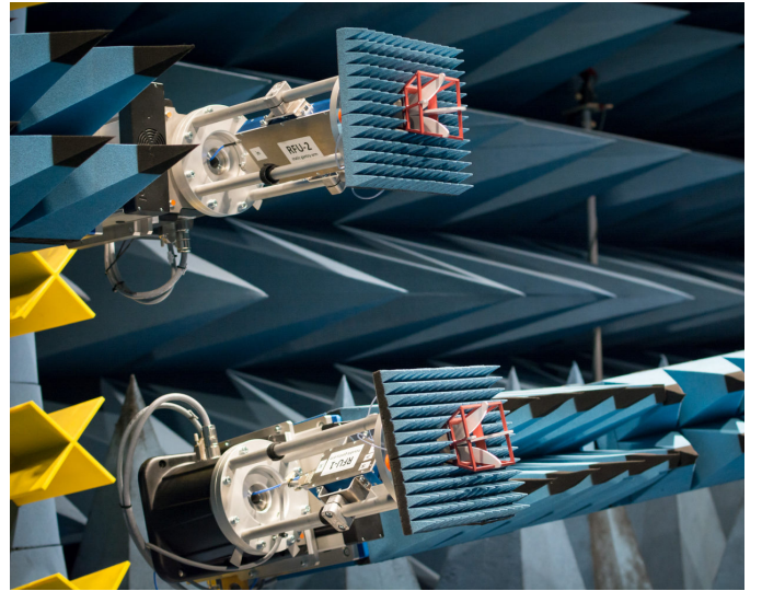
Fig. 4. Non-converting microwave probes at tip of both gantry arm positioners: Tx and Rx amplifiers, RF switches for polarization, and RFspin QRH20E dual-polarized antennas surrounded by absorbers. This configuration is used for VNA measurements of static targets. See Table II for technical details.
