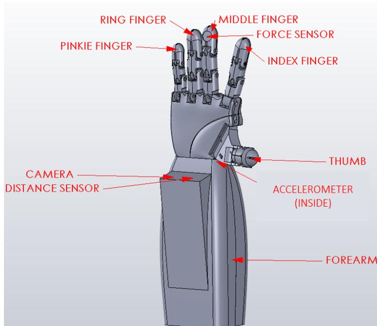
Figure 2: 3D Design of Vision-Enabled Sensorized Prosthetic Hand
