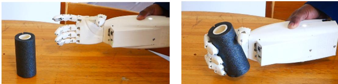
Figure 5: Grasping the object with the prosthetic hand
